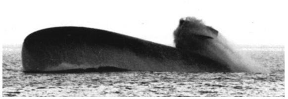
The USS Philadelphia "breaching" after a test of its emergency blow system. The emergency blow system is designed to rapidly empty the sub's ballast tanks and in doing so, force the sub to the surface.
