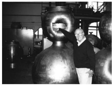
John Murphy in the area of the Krylov Institute submersible laboratory where submersibles undergo pressure testing to determine the maximum survivability for submarines and research vessels at deep ocean depths. Murphy explains, "If it bursts, we have failed!"
